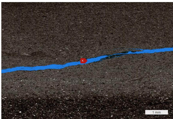
K - Induced fracture locally filled with rock flour (dark-colored material on the right) associated with sample drilling or trimming
