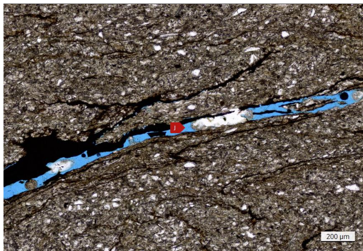
J - Induced fracture; the white area on the right is an air bubble associated with blue epoxy impregnation
