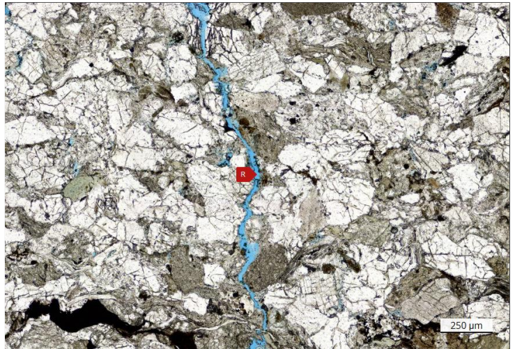
R - Induced fracture
