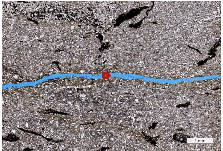
J - Sampling-enhanced microfracture
