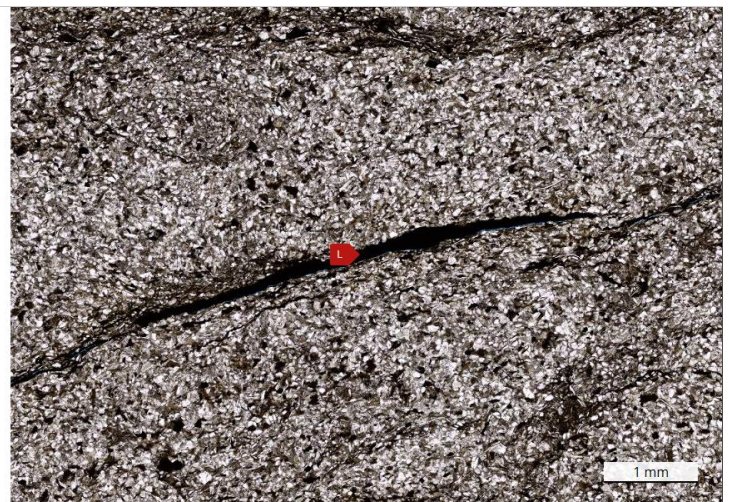
L - Elongate organic fragment; partly replaced by authigenic pyrite
