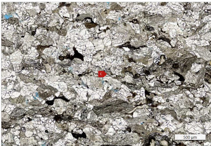
C - Stylolite highlighted by the concentration of clay, organic matter and other insolubles
