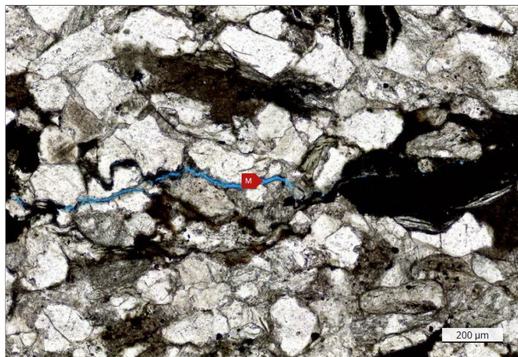
M - Induced fracture
