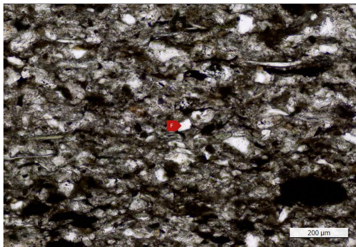
F - Silt-size detrital quartz grain
