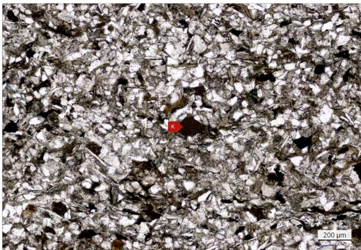
K - Siderite-replaced grain
