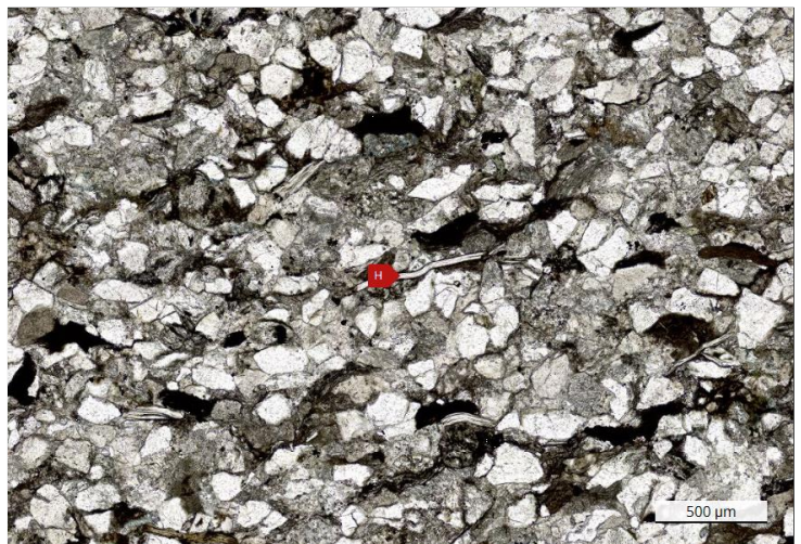
H - Detrital muscovite mica grain; slightly deformed due to compaction
