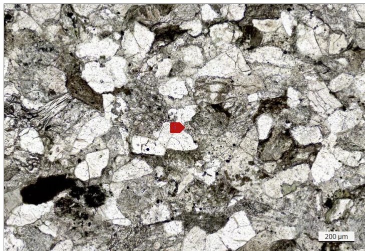
I - Carbonate cement filling intergranular areas
